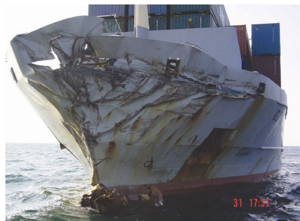
Fig.10. The bow damage of container ship after collision [14]
