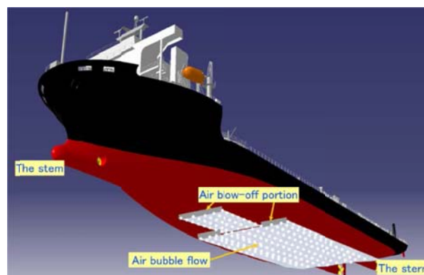
Figure 3. Mitsubishi air lubrication system
