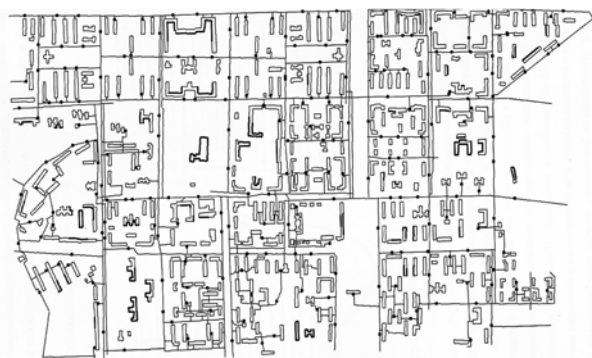
Fig. 6. Placement of fire hydrants (dots on the water supply network) in Ordzhonikidzevskiy area of Kharkov, Ukraine
