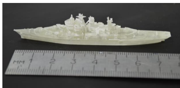
Fig. 8 3-inch long 3D printed ship [6]
