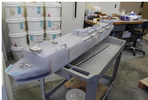
Fig.20. 3D printed model of hospital ship USNS Comfort (T-AH20) [24]
