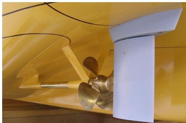
Fig. 19. 3D printed rudder in model basin HSVA [23]
