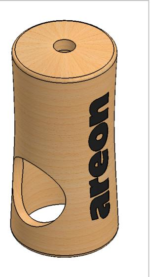
Non-prescribed limit deviations of the dimensions are: ± IT14 / 2. Traces, flips of machining and scratches on the outer cylindrical surface of the body are not allowed. The logo is hot stamping, bilateral 0,15mm minimum depth, and it is by our design.
